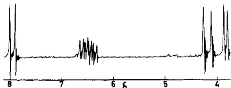
Figure 3. The ^1\text{H} NMR spectrum of vinyl alcohol under conditions where exchange of the hydroxyl proton is slow; it was generated from 8 in \text{CD}_3\text{COCD}_3 (99 v %)/ \text{H}_2\text{O} (1 v %) which contained 10^{-4} M HCl at -10^\circ\text{C} .
